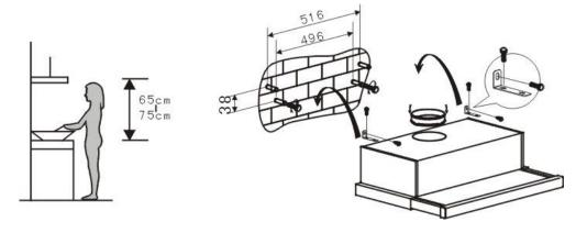
**Step 6:** Fix the rangehood onto the wall, like demonstrated in the above picture.
