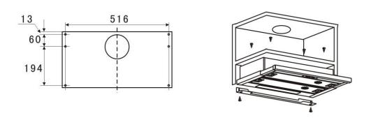
**Step 1:** The rangehood should be placed at a minimum distance of 65cm above the cooking surface when placed above an electric hob and a minimum of 75cm above the cooking surface when placed above a gas cooktop.
